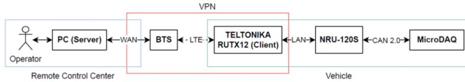
Fig. 1. Proposed Remote Control Architecture
