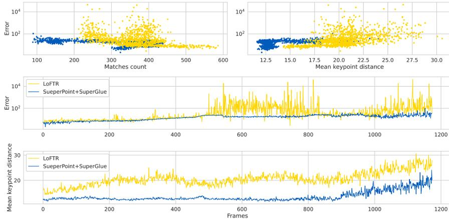
Fig. 2: 2D Error in meters related to the number of good matches and mean keypoint distance for SuperPoint with SuperGlue and LoFTR.
