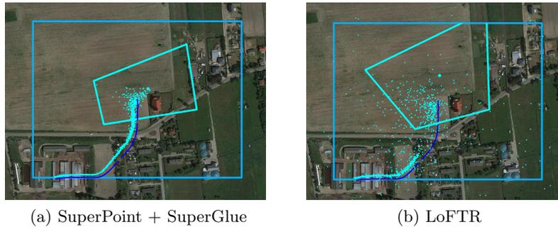
Fig. 1: Visual comparison of image-based localization methods. Large rectangle is ROI used for localization. GPS trajectory in dark blue. Points in cyan - localization result. Cyan quadrilateral - represents field-of-view of the localized camera.
