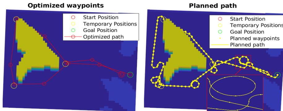
**Fig. 2.** Sample output of APP: global waypoints (left) and concatenated local path (right)
