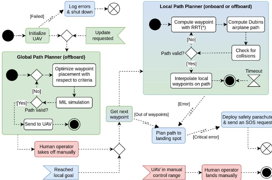
**Fig. 1.** A typical HALE UAV measurement mission using APP
